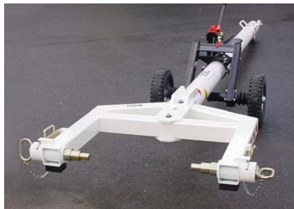
Tow Bar fitted with the adapter-head for DC8 aircraft.
