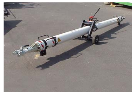
This adapter-head can be used for different aircraft such as Tu154, IL96 and BAE 146.
