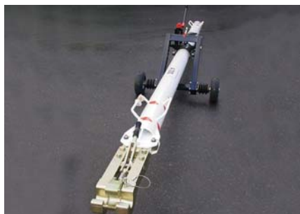
An adapter-head for the Airbus 330 mounted on a standard tow bar.
