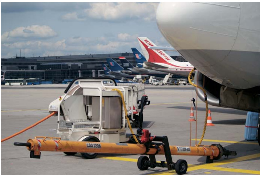
A Cavotec Fladung tow bar connected to a tow truck at Frankfurt Airport, Germany.
