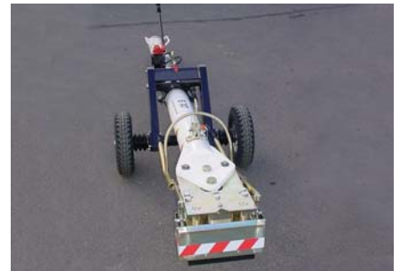
A Boeing 747 adapter-head fitted on a steel tube with floating axle.
